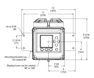
4x M8 x 16 bolts are included for attaching the mounting bracket to the Model 3350 or 3700 transmitter
