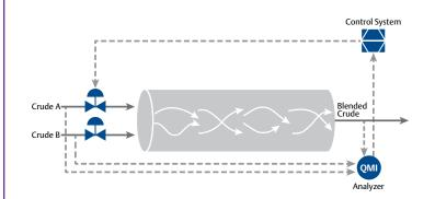
Feed Forward and Feedback Control allows you to accurately blend to the TBP curve for optimal crude unit utilization. ▶ p15-16
