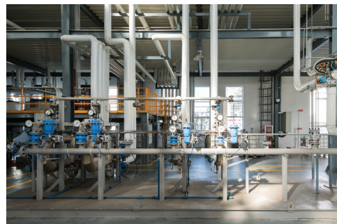
A 4-Loop Simultaneous Metered Blender with piggable discharge header installed in China. Photo courtesy of Copton.
