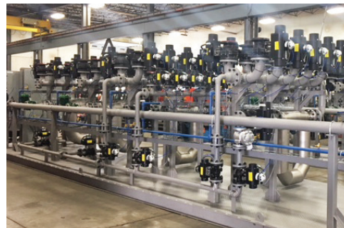
Turnkey Simultaneous Metered Blender undergoing Factory Acceptance Testing.
