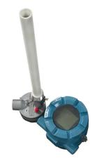
so that both its oxygen probe and the electronics are intrinsically safe without requiring costly design modifications such as flame arrestors. The oxygen probe is constructed of ceramic materials capable of withstanding high process temperatures. Also, the analyzer eliminates the use of the cell heater, using the higher process temperatures to heat the zirconium oxide sensor cell to the temperature required by the Nernst equation principle of operation.
