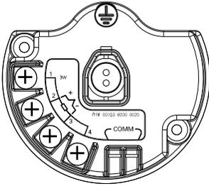
Figure 2. Rosemount 648 Wireless Sensor Connections
